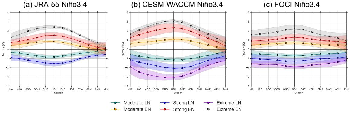
**Figure S6:** Composited 3-month average seasonal evolution of the Niño3.4 SSTA (in K) for JRA-55 (a, 1958-2021) and the ensemble means for CESM-WACCM (b), and FOCI (c). Events are subsampled into moderate, strong, and extreme events, as outlined in the methods. Shading represents the 95% confidence interval, while the solid line represents the mean.
