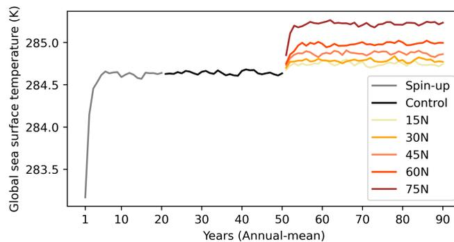
**Figure S2.** The temporal evolution of global, annual mean sea surface temperature (K) in the periods of spin-up (years 1 to 20), control (years 20 to 50) and the perturbation experiments (years 50 to 90). The perturbation experiments are branched off from the last day of year 50 from the control experiment. The first 10 years (years 50 to 60) from the perturbation experiments are discarded.
