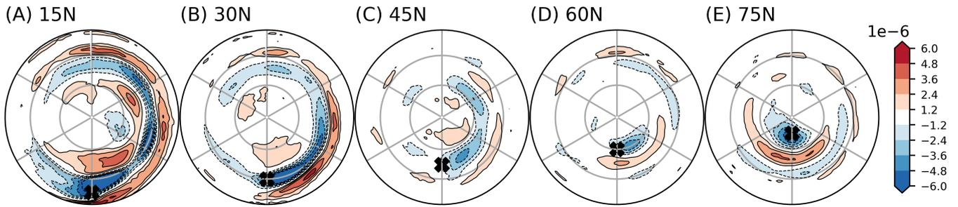
**Figure S5.** Upper level (232 hPa) vorticity response ( $\text{s}^{-1}$ ) in the (A) 15°N, (B) 30°N, (C) 45°N, (D) 60°N and (E) 75°N heating perturbation experiments. The crosses mark the position of the surface heating perturbation. The latitude lines mark 30°N and 60°N. The longitude lines denote 60° intervals, marking 120°W, 60°W, 0°, 60°E, 120°E and 180°.
