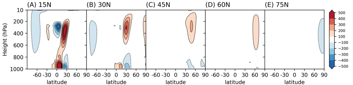
**Figure S4.** Meridional heat transport response ( $\overline{vT}$ ,  $\text{Kms}^{-1}$ ) in the (A) 15°N, (B) 30°N, (C) 45°N, (D) 60°N and (E) 75°N heating perturbation experiments. The latitude-height section is shown as the zonal average over the longitudes of the Q-flux perturbations.
