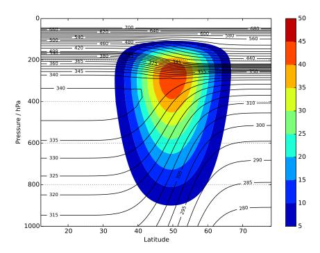
Figure 1. Initial potential temperature and U wind using setup according to Baker et al. (2014) but with  $m_v = 10^{-8}$  in the stratosphere and  $\Gamma_S = 0.025$ , profile correction option 2. Note  $\theta$  contour interval changes from 5 K to 20 K at 400 K.
