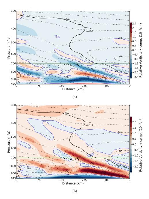
Figure 8. Cross sections on transect CD of Fig. 5a of (a) zonal and (b) meridional components of relative vorticity (shading),  $\theta_w$  (thin black dashed contours, K) and cloudy regions (RH<sub>ice</sub>=80%, black bold contours) at 83 hours from run start. Black dots show the perpendicular projection on the transect of the trajectories that are less than 25 km distant from the relevant transect. The green line indicates the pressure of 700 hPa, to which Figure 6a refers.
