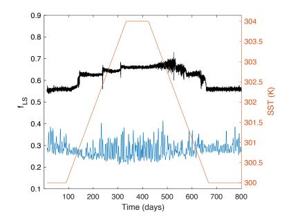
**Figure 4.** Left axis:  $f_{LS}$  for the WRF SCM over 800-day RCE (blue) and WTG (black) experiments. When running the SST-forcing experiment in a RCE configuration, the unfiltered  $f_{LS}$  has an average value of ~0.28 and a standard deviation of ~0.18. (The presented RCE  $f_{LS}$  data have been low-pass filtered for clarity.) Right axis: SST over the experiments.
