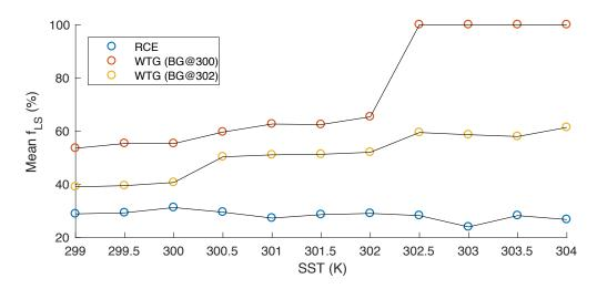
**Figure 3.** Average  $f_{LS}$  for the last 15 days of a series of 30-day RCE experiments and two series of WTG approximation experiments with different background profiles, one equilibrated to a SST of 300 K and another to a SST of 302 K. In the case of the WTG experiments using the 300 K background profile, the last four experiments demonstrate the fact that  $f_{LS}$  can go to unity in some cases.
