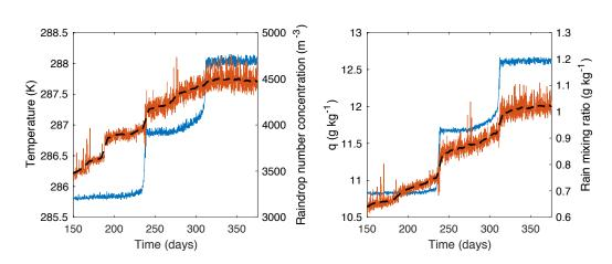
Figure 10. Potential precursor activity for the second and third abrupt transitions. (Left panel) Left axis: temperature (T) evolution (blue). Right axis: raindrop number concentration evolution (red) with low-pass filtering shown in black. (Right panel) Left axis: water vapor mixing ratio (q) evolution (blue). Right axis: the rain water mixing ratio evolution (red) with low-pass filtering shown in black. All quantities are at  $p \approx 835$  mb.
