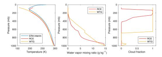
**Figure 1.** Left: Tropical soundings from ERA-Interim reanalysis (observational) data and averages over the last 30 days of two 180-day WRF SCM experiments, one a RCE experiment and one with the WTG approximation active both with fixed 300 K SST. Center: Water vapor mixing ratio profiles from the same RCE and WTG experiments. Right: Cloud fraction profiles from the same RCE and WTG experiments.
