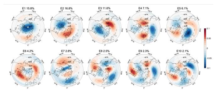
Figure 1. The first 10 EOF spatial patterns of PV at 850 K ( $E_1, E_2, ..., E_{10}$ ) of the combined set of basis vectors as described in the text using ERA-Interim daily data. The percentage number indicates the variance explained by each EOF.
