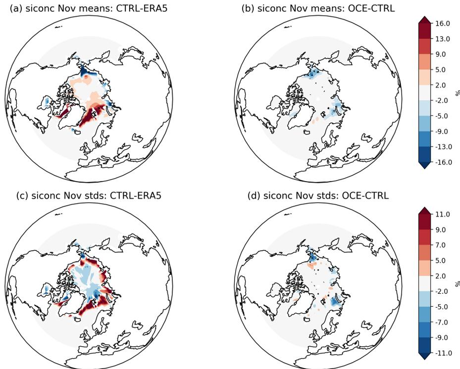
**Figure 1.** Sea ice concentration (mean and standard deviations) in November. Mean quantities in (a) CTRL-ERA5 and (b) OCE-CTRL. Standard deviations in (c) CTRL-ERA5 and (d) OCE-CTRL. Stippling in (b) and (d) highlights gridpoints where the change is statistically significant ( $p < 0.05$ ); in (a) and (c) almost every gridpoint outside the zero contour is significant so stippling is not included for visual ease. The period considered is 1980-2015.
