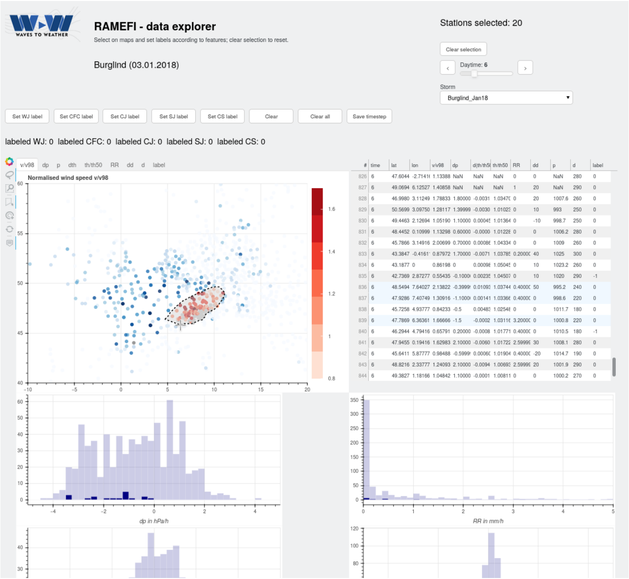
Figure D1. Screenshot of the interactive visualisation and labelling tool as part of RAMEFI (Eisenstein et al., 2022a) using the Python package bokeh (Bokeh Development Team, 2021). The user can switch between timesteps and loaded winter storms. Top row shows a map of stations and their parameters, here \tilde{\omega} , where the user can select an area by mouse using a lasso or clicking on single stations. Labels for the introduced features can be set for the selected stations. A table includes all data points and parameters. Histograms are shown for several parameters for the whole region (light blue) and currently selected stations (dark blue).
